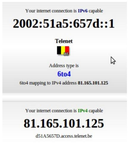
Going to the test-ipv6.com website will also test whether you have a valid accessible ipv6 address.
