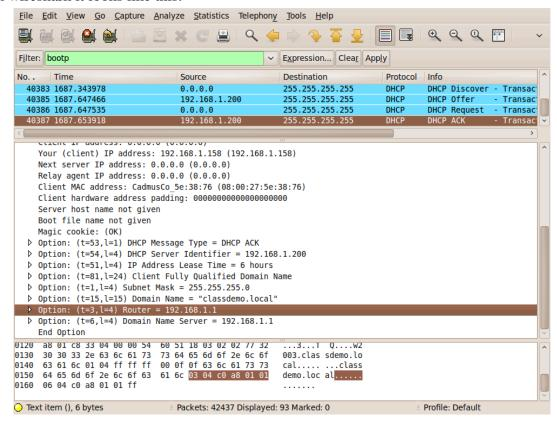
When this procedure is finished, then the client is allowed to use that ip-configuration until the end of its lease time.
