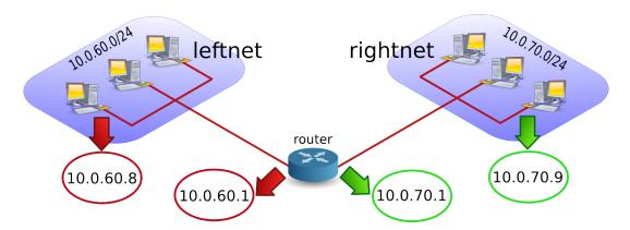
2. Set up a third Linux computer with three network cards, one on **leftnet**, the other on **rightnet**. This computer will be the 'router'. Complete the table below with the relevant names, ip-addresses and **mac-addresses**.
