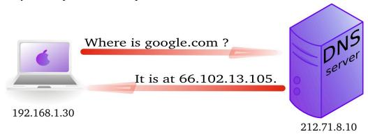
In wireshark you can use the **dns** filter to see this traffic.
