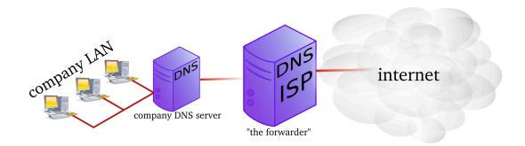
This picture shows a **dns server** on the company LAN that has set the **dns server** from their **isp** as a **forwarder**. If the ip address of the **isp dns server** is 212.71.8.10, then the following lines would occur in the **named.conf** file of the company **dns server**:
