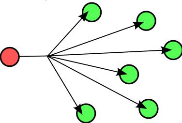
Typical example here is the BBC (British Broadcasting Corporation) broadcasting to everyone. In datacommunications a broadcast is most common confined to the **lan**.
